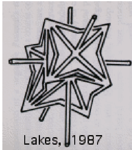
Fig 1.6 Idealized re-entrant unit cell produced by symmetrical collapse of a 24-sided polyhedron with cubic symmetry [1]
