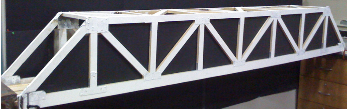
Fig 3.2 Picture of the actual model wood bridge
